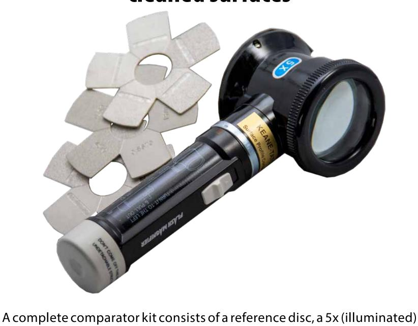
magnifier with magnetic disc holder, and a viny disc case. REFERENCE DISC DESCRIPTION
