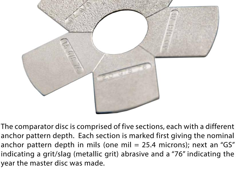
year the master disc was made. **HOW TO USE** Determine the profile of metallic grit blast cleaned steel by choosing the reference disc segment that most closely approaches the roughness of the blast. Note that roughness may lie between two segments and
